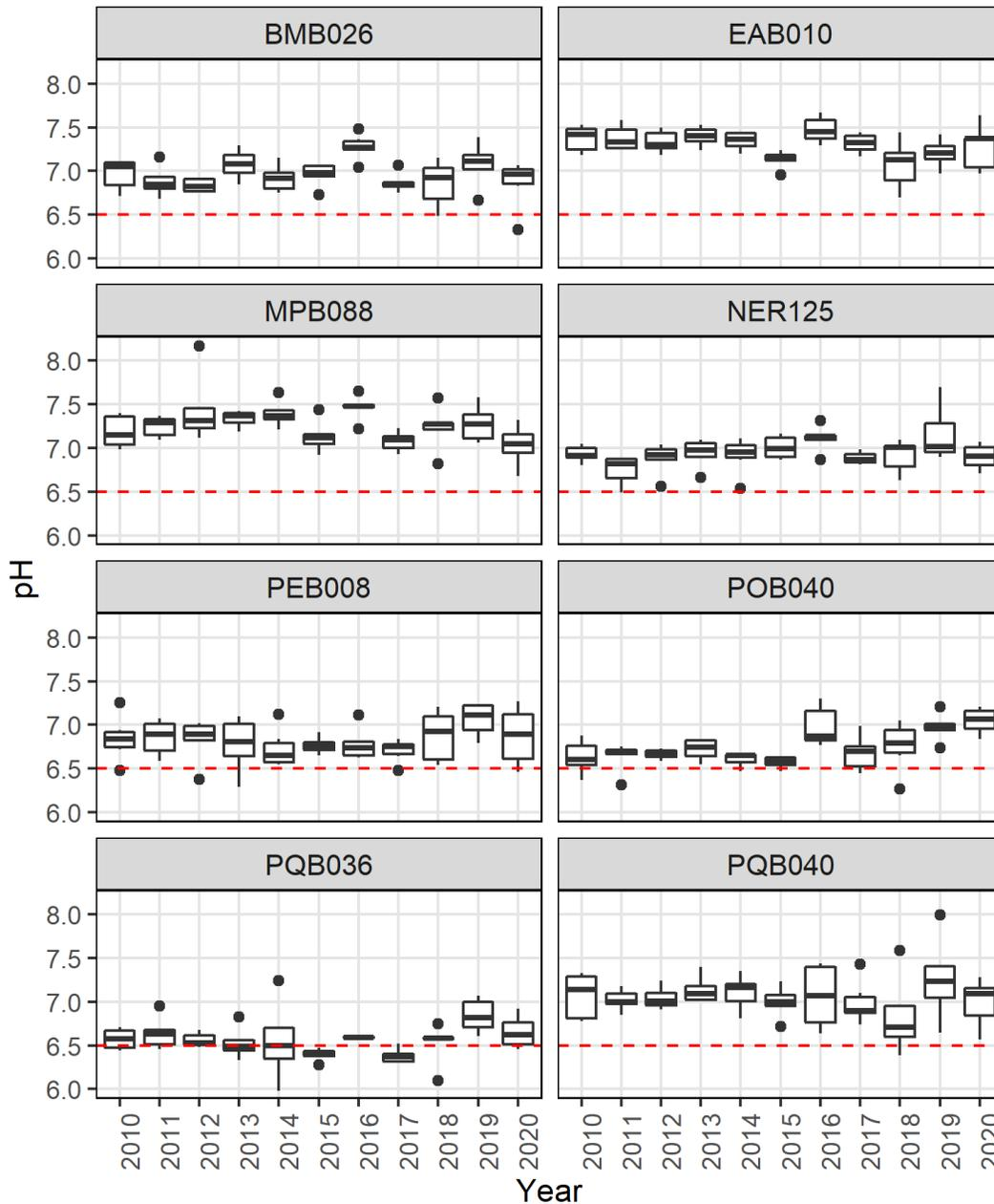
Figure 5: The pH levels at the eight sites in Canton for years 2010 through 2020. Boxplots statistics are the same as Figure 2. The red dashed line is at pH = 6.5, the lowest allowable pH level in Massachusetts.
