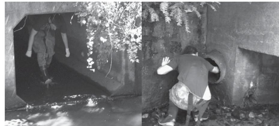
Intern Joe MacDonald worked with NepRWA Environmental Scientist Bill Guenther over the summer to locate illicit connections in the Neponset River Watershed. Here, Joe sets up optical brightener tests inside pipes on Unquity Brook in Milton. The tests will help to locate any sources of untreated wastewater and sewage pollution.
