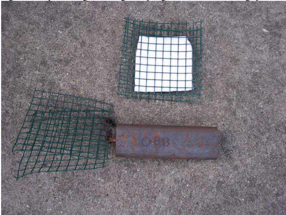
Figure 10: Optical Brightener cage sampling device with anchoring system attached.
