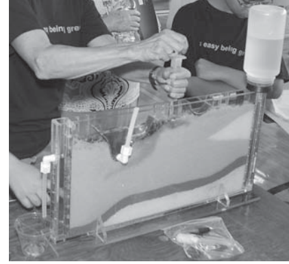
Demonstrating the flow of water and pollutants through the ground with a groundwater model.
